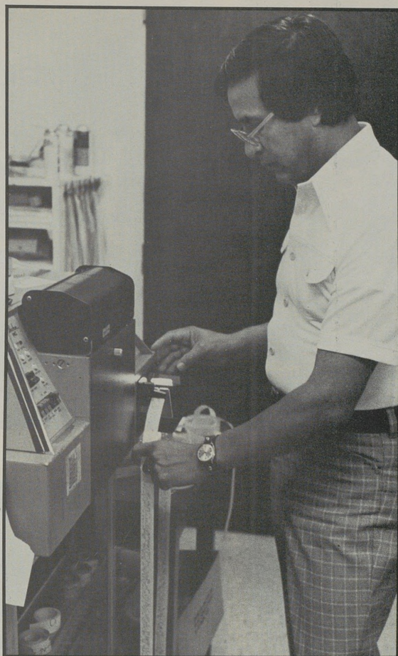
Above: Typesetter punches tape for an article. Right: Tape is converted into camera-ready copy for magazine layout.
