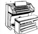
NEW Model 2C: Two 61-note manual keyboards; full 32-note pedal board. A. G. O. specifications.
