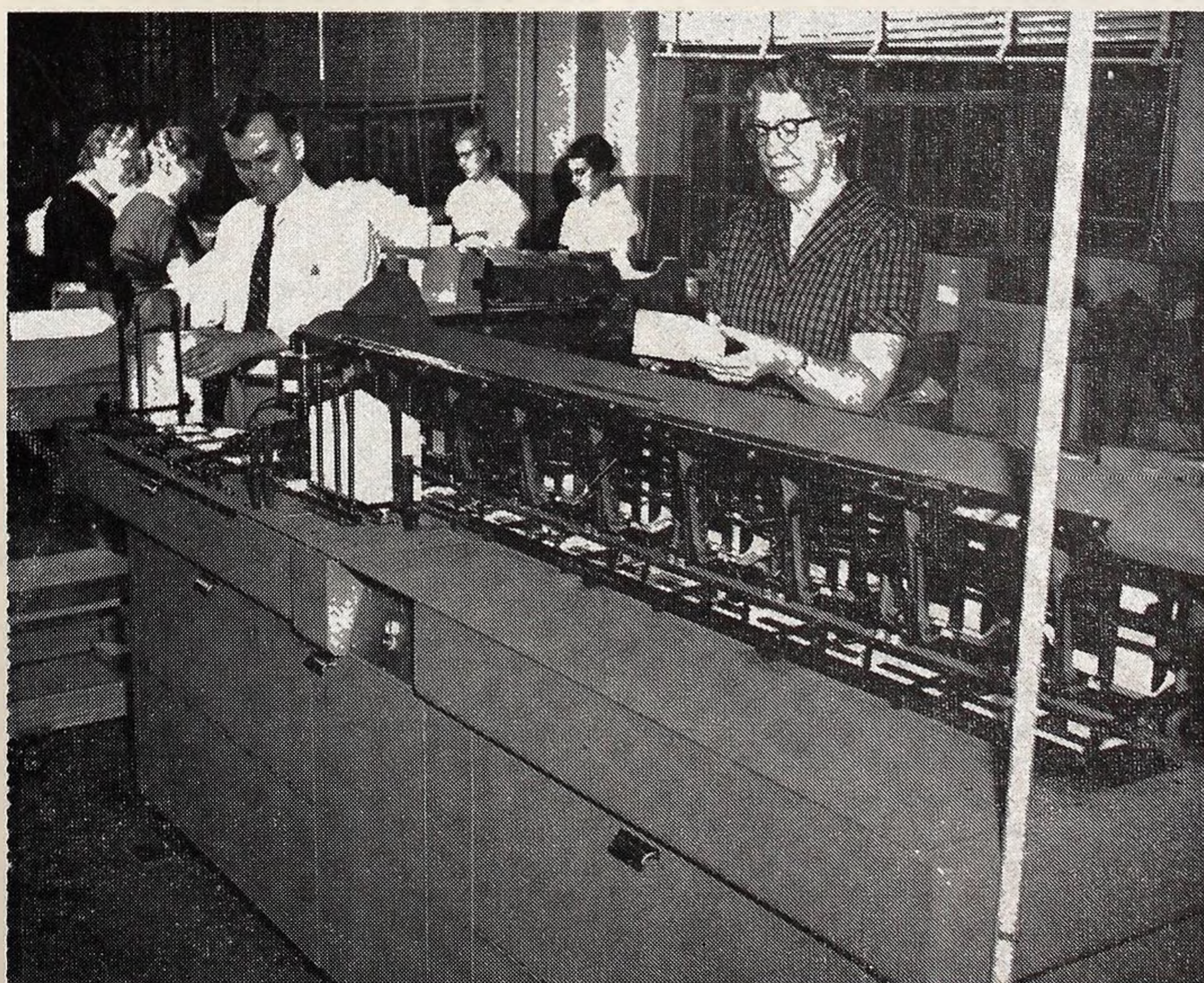
NASHVILLE—The Sunday School Board of the Southern Baptist Convention has put into use this ultimate in the way of inserting and mailing machine. Work requiring five persons three days can be done by this machine and one operator in one eight-hour day. It has been installed to reduce operating costs, to speed up service to Southern Baptist churches and maintain mailing schedules. Tommy Grubbs and Mrs. Sudie Summers, employees of the Board, are shown with this new "robot" inserting and mailing machine which is said to be the largest in the southeast.
